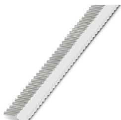
Taped ferrules, 0.5 mm<sup>2</sup>, sleeve length 8 mm, with plastic collar, according to DIN 46228-4, white, for processing with the CRIMPFOX 4 IN 1, 10 strips each with 50 sleeves per strip.
