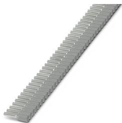
Taped ferrules,  $0.75 \text{ mm}^2$ , sleeve length 8 mm, with plastic collar, according to DIN 46228-4, gray, for processing with the CRIMPFOX 4 IN 1, 10 strips each with 50 sleeves per strip.
