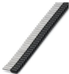
Taped ferrules,  $1.5 \text{ mm}^2$ , sleeve length 8 mm, with plastic collar, according to DIN 46228-4, black, for processing with the CRIMPFOX 4 IN 1, 10 strips each with 50 sleeves per strip.
