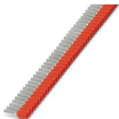
Taped ferrules,  $1.0 \text{ mm}^2$ , sleeve length 8 mm, with plastic collar, according to DIN 46228-4, red, for processing with the CRIMPFOX 4 IN 1, 10 strips each with 50 sleeves per strip.
