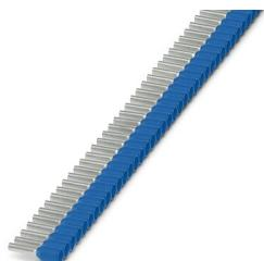
Taped ferrules,  $2.5 \text{ mm}^2$ , sleeve length 8 mm, with plastic collar, according to DIN 46228-4, blue, for processing with the CRIMPFOX 4 IN 1, 10 strips each with 40 sleeves per strip.
